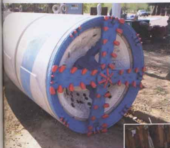
Above: Sharp end of the Akkerman microtunneling machine
