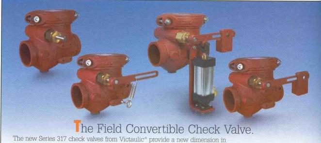
service and adaptability. Grooved ends reduce the weight of the valve making it faster and easier to install. A closure coupling and cap give you quick access to the valve for any required maintenance. This AWWA C-508 valve features a clear flow design and offers positive sealing in either a horizontal or vertical position for pressures up to 175 psi. All accessories are designed for direct mounting in the field.
